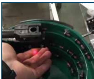
Screw feeder with 'over-unloaded' sensor for activation of screw feed
