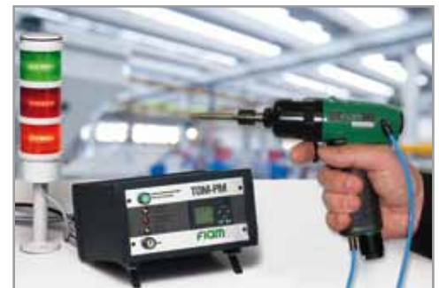
Models with pneumatic pick-up signal (ported) for screw counting (poka yoke system) available upon request
